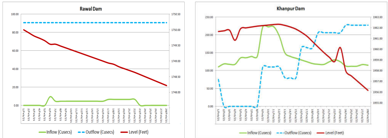
Figure 8: Water inflow, outflow and level of Rawal and Khanpur Dams
